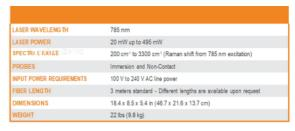
Tornado's HyperFlux™ PRO Plus is a complete Raman spectroscopy system including a proprietary HTVS™-enabled spectrometer, a high-quality stabilized laser, multiple laser safety interlocks, temperature monitoring and dynamic re-calibration, and automated system health monitoring and fault detection.
